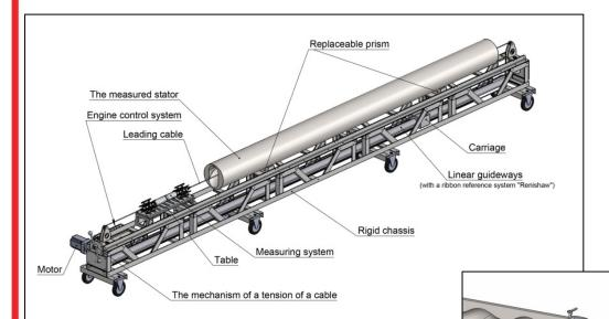
**Designed use:** Progressive cavity stators, tubes and pipes, gun barrel bore (rifled and smooth)
